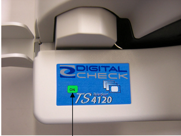
Fig. 6: The left LED comes on 'Red' to indicate power to the unit. When the scanner is acquired by the application, the left LED turns 'Green'.
