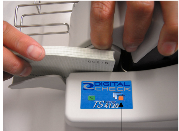
Fig. 7: The right LED is the document in pocket indicator after acquisition.
